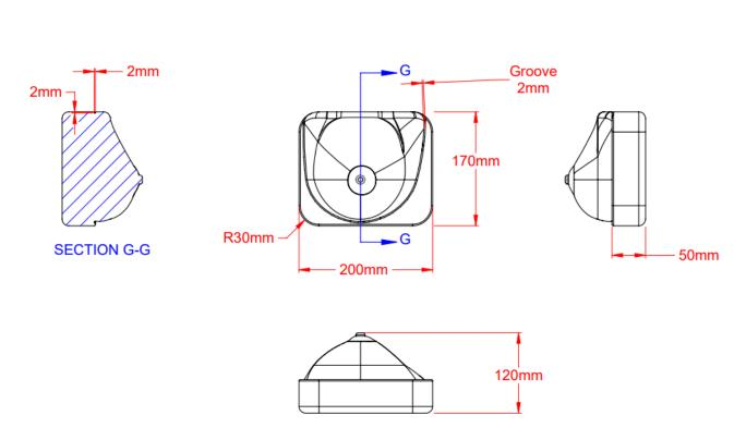
FIGURE 3: Drawing – Dimensions of the Very Large Breast Phantom
